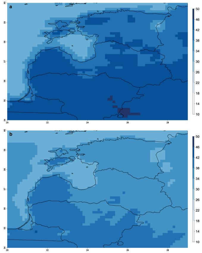
**Fig. 4** Mean amount of low clouds (%) **a** in autumn (SON), **b** in winter (DJF), **c** in spring (MAM) and **d** in summer (JJA) during the period 2008–2013. Data obtained from the SEVIRI instrument onboard the MSG satellite with a spatial resolution of  $15 \times 15$  km
